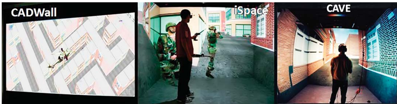
Fig. 8. Integrated Visualization Platform—left: 4-wall large-screen data wall at daytaOhio, a 4-wall immersive facility at Wright State University, and a 5-wall immersive facility located in AFRL's Battlespace Acoustic Branch; middle: multimodal display systems including stereoscopic visualizations, 3-D audio and haptic/tactile displays; right: research platform designed for evaluating the effectiveness of advanced displays and technologies in operationally-relevant scenarios.
