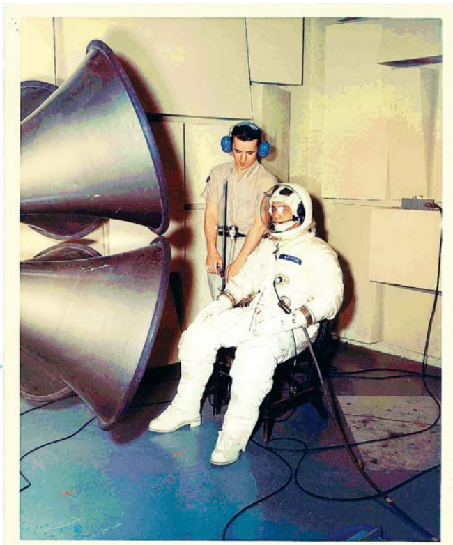
Fig. 2. High intensity noise test at AFRL, circa 1960.
