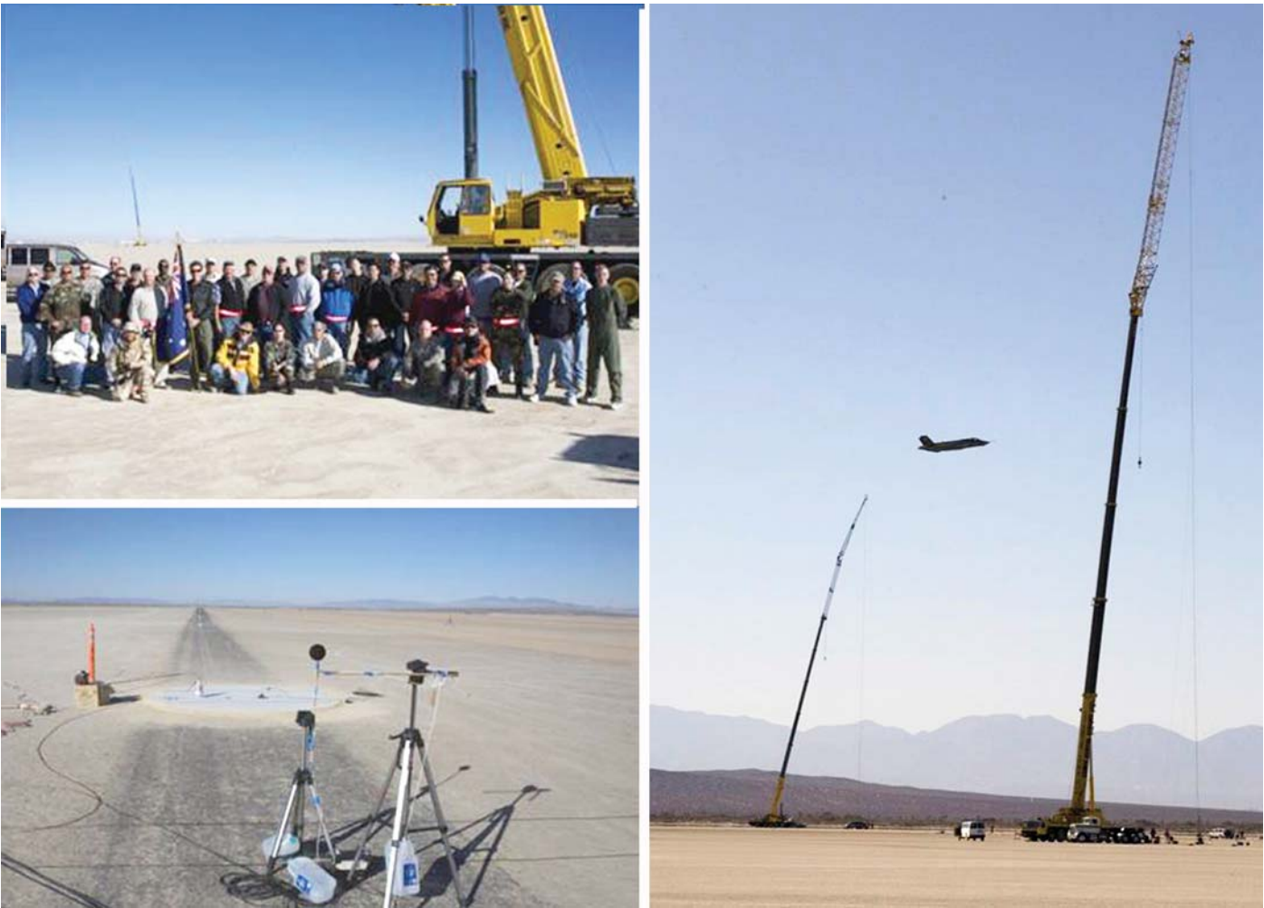
Fig. 10. F-35 Lightning II, flyover noise measurement—clockwise from upper-left: the crew; flyover and tower sensors; ground sensors.
