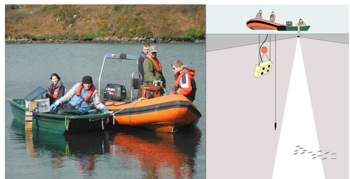
Figure 3: Sound playback experiments were carried out from two boats, tethered together, drifting silently over fish schools. An array of four low frequency sound projectors was suspended from one boat, and a sonar system on the second boat used to observe fish schools. A short sequence of impulsive sounds (simulating percussive pile driving sounds) was transmitted and the subsequent responses of the fish followed on a combined echo sounder and side-scan sonar. A hydrophone was subsequently deployed at different depths to measure the received sound levels.
