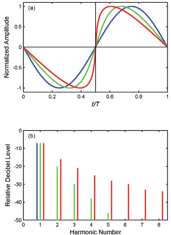
Fig. 2. a) Graph of normalized acoustic amplitude as a function of  $t/T$  at three propagation distances. The initially-sinusoidal waveform is depicted in blue. The green and red curves show the waveform at successively greater propagation distances, respectively. The waveform becomes more and more distorted as it propagates. b) Graph of the frequency spectrum of the waveforms shown in a). Increased waveform distortion is accompanied by increased harmonic content.
