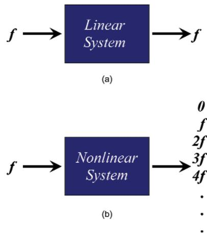
Fig. 3. a) A stimulus of frequency  $f$  applied to a linear system results in an output at, and only at, the same frequency  $f$ . b) In contrast, a nonlinear system responds to an input of frequency  $f$ , with an output consisting of harmonics of  $f$ .
