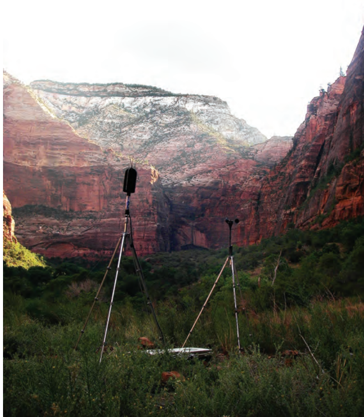
Fig. 1. A National Park Service (NPS) acoustical monitoring system deployed in Zion National Park. Through many generations of NPS systems, wind speed logging has been a consistent component, to identify times when pseudonoise generated by airflow around the wind screen would inflate the spectrum measurements.
