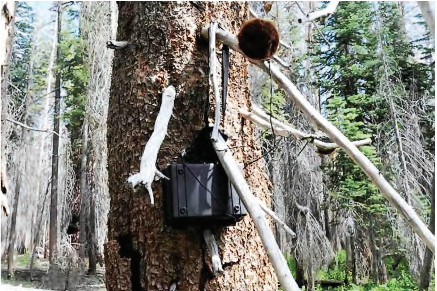
Fig. 4. The recording system utilized by Joe Medley (U. C. Davis) to monitor great grey owls in the Sierra Nevada mountains of California. Two preamplified electret microphones (SuperCircuits PA3) were inserted into the throats of laboratory funnels, which served as conical horns. The rectangular case contained rechargeable NiMH D cells and a Cowon iAudio 7 solid state recorder.
