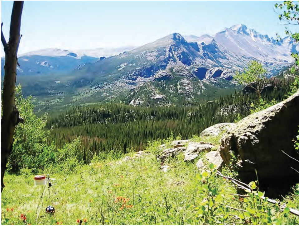
Fig. 3. National Park Service (NPS) landscape scale soundscape survey in Rocky Mountain National Park. This system utilized a digital audio recorder (Zoom H2) and relied upon its internal microphones. The electronics were protected underneath an enclosure that served as both a wind fairing and weather protection.
