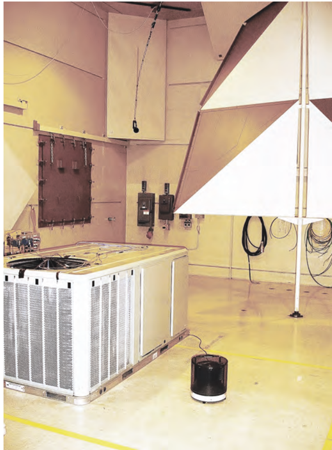
Fig.1. Qualified reverberation room with system ready for sound power measurements.
