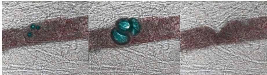
Fig. 5. A group of bubbles distends the vessel wall (middle) during the tensile portion of the sound wave; subsequent invagination (right) appears localized and markedly larger than the distention. Time stamps are, from left to right, 1.3, 1.6, and 3.4 \mu\text{s} after arrival of a 2-cycle ultrasound pulse of amplitude 6.4 MPa. Vessel diameter is approximately 46 \mu\text{m} . Images were colored
