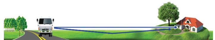
Figure 5. Highway traffic noise propagation – direct and ground-reflected sound. Illustration modified from Highway Traffic Noise , National Highway Institute (NHI) course 142051.
