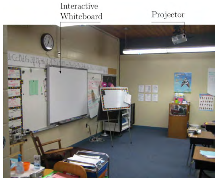
Figure 4. Many classrooms still use video projector technologies. This is an example of a typical interactive whiteboard that uses a video projector. Video projectors can contribute to the BNLs that teachers must compete against.
