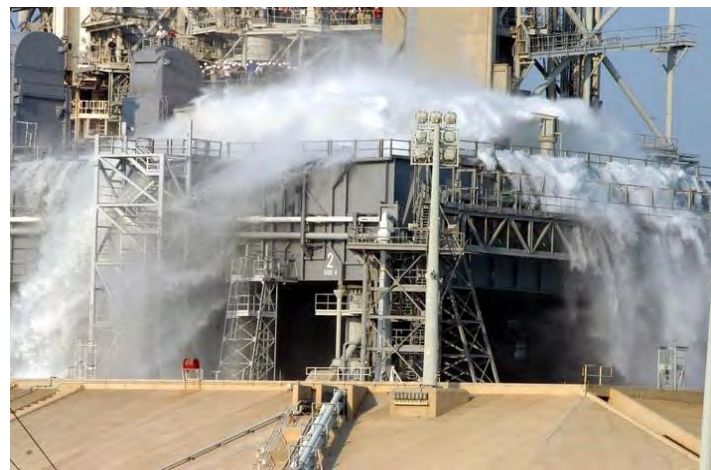
Figure 3. Water from an acoustic suppression system test soaks the mobile launcher platform at the Kennedy Space Center Pad 39A with 350,000 gallons of water. Photo available at bit.ly/2P1W93e .
