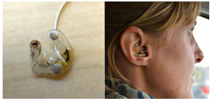
Figure 4. Example of an in-ear electroencephalographic (EEG) mount shown as a single earplug (left) and in the ear (right). Own work by Mikkelsen.kaare, Creative Commons Attribution-ShareAlike 4.0 International Public License (CC BY-SA 4.0). commons.wikimedia.org/w/index.php?curid=51268329 .
