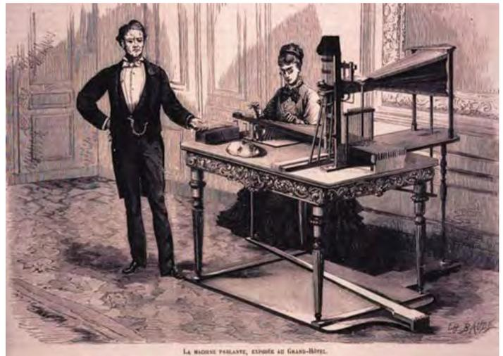
**Figure 6.** Faber’s “Euphonia,” exhibited at the Grand Hôtel in Paris in 1877 by his niece and nephew-in-law. This is one of the few illustrations of the whole speaking machine, showing the bellows driven by a foot pedal, the box containing the mechanism shown in **Figure 5**, and the system of rods and levers linking the different articulators to the keyboard. Reproduced from *L’Illustration* (January 1877).
