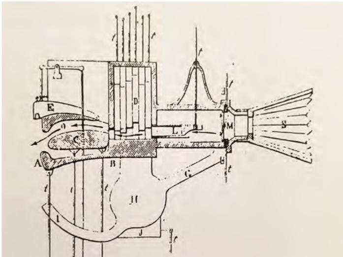
**Figure 5.** The mechanism of Faber’s “Euphonia,” illustrated by du Moncel (1882), showing the bellows (S), the vibrating reed (L), the trill mechanism (M), the moving blocks (D), the jaw (A and B), the tongue (C), the palate (E), the nasal cavity (G, H, and I), and the levers (t) connected to the keyboard; **arrows** indicate the direction of airflow. Reproduced from du Moncel (1882).
