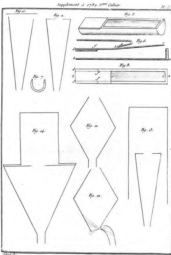
**Figure 2.** Kratzenstein's five vowel tubes for the vowel sounds *a* (two cross sections in Figs. 9, 10), *e* (Fig. 11), *i* (Fig. 12), *o* (Fig. 13), and *u* (Fig. 14), excited by a free reed (Figs. 5-8). Kratzenstein remarks that the passage from *o* (Fig. 13) to *u* (Fig. 14) is achieved by the stricture of the upper cavity. Reproduced from Kratzenstein (1780).
