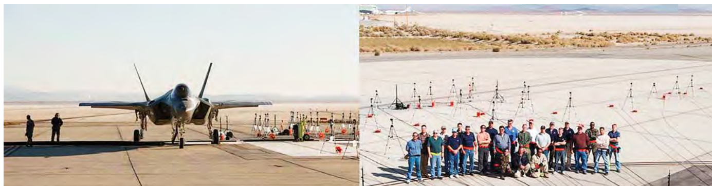
Fig. 9. F-35 Lightning II (Joint Strike Fighter), ground run-up noise measurement—left: the aircraft; right: the crew and some of the near-field sensors
