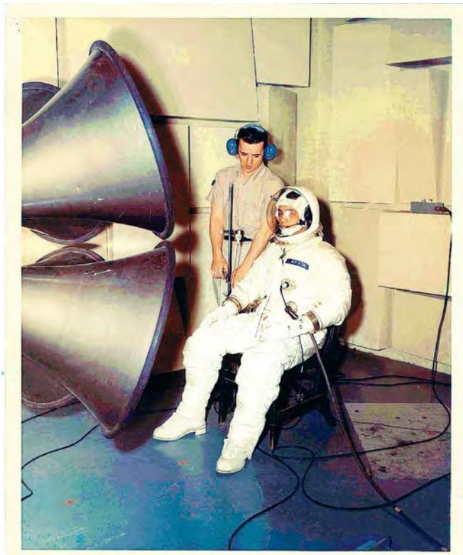
Fig. 2. High intensity noise test at AFRL, circa 1960.
