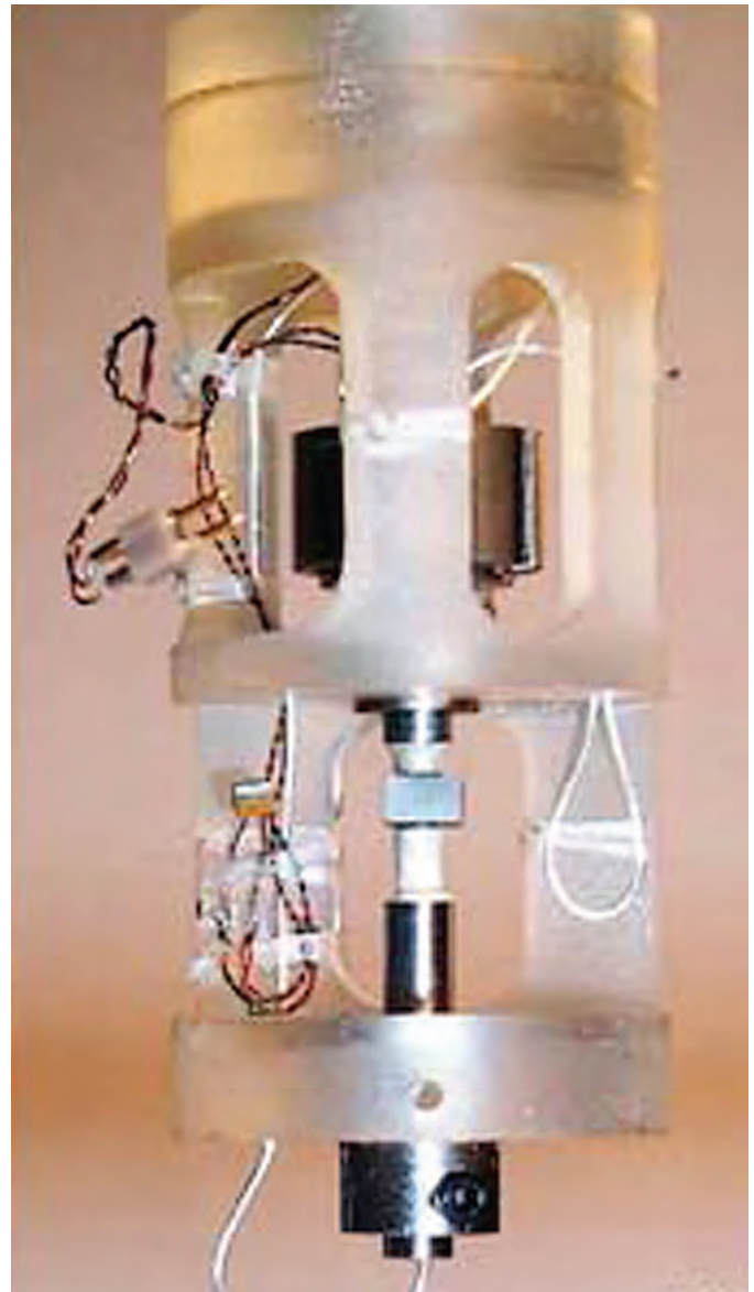
Fig. 2. Resonant Ultrasound Spectroscopy probe for measurements at low temperatures and in high magnetic fields.
