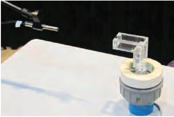
Figure 7. Experimental set-up for making recordings using bent-type models with sliding blocks (Models A and B)
