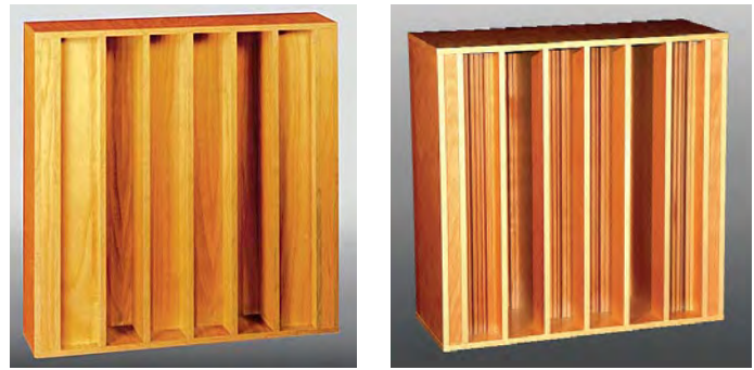
Fig 4. One period of two different Schroeder diffusers. Left—original design, right—fractal design. The diffusers are 0.6m wide, 0.6m high and about 0.2m deep.
