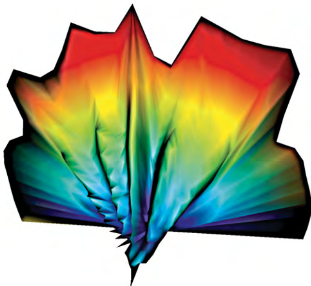
Fig 8. Scattered pressure level from a modulated, optimized, reflection phase grating.
