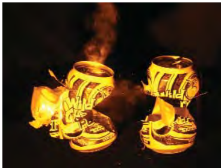
Ping-pong ball driven by atmospheric pressure passes through two soda cans following explosive shock heating. (Photo by Tom Rossing.)
