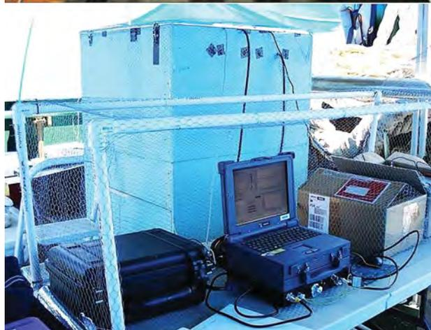
Fig. 5. Field portable system developed at Space and Naval Warfare Systems Center (SSC) San Diego consisting of bioamp (in Pelican case, bottom photo, shown with system running onboard a ship), ruggedized computer with data acquisition hardware, and Evoked Response Study Tool (EVREST) software developed by J. J. Finneran for generating sound stimulus signal, recording and storing auditory evoked potentials (AEPs), and analyzing data.
