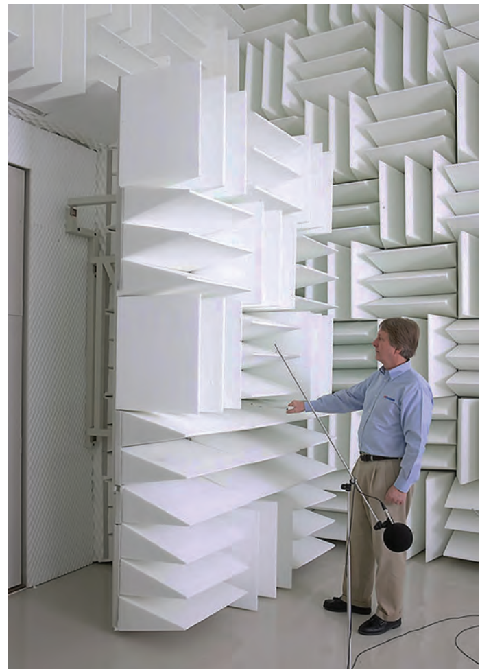
Fig. 9. One wedge basket door in operation.
