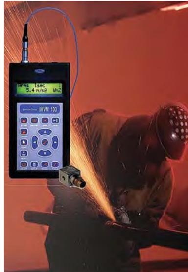
The Larson Davis division of PCB Piezotronics (PCB®) has announced the launch of a new series of high performance triaxial accelerometers, Series SEN04xF, designed expressly for taking measurements of worker personal exposure to Hand-arm Vibration (HAV). Designed with special integral low-pass filtering circuits that minimize false readings from shock and mechanical resonances, Models SEN040F (1 mV/g sensitivity) and SEN041F (10 mV/g sensitivity) are smaller, lighter
