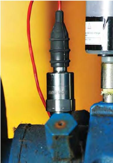
The IMI Sensors division of PCB Piezotronics (PCB®) has released Series 686B USB Programmable Smart Vibration Switch, designed for 24/7 continuous monitoring and protection of cooling towers, fin fans, pumps, HVAC systems, and other critical machinery. This electronic switch has much better accuracy and reliability than traditional mechanical switches, and is easily installed in
