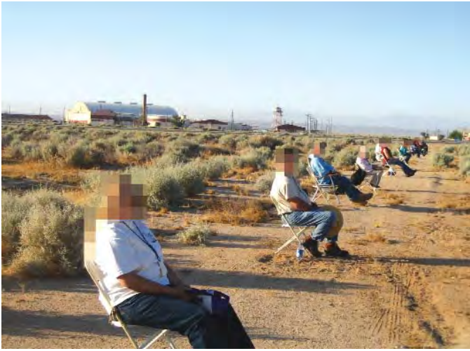
Fig. 7. Jury testing participants listen to sonic booms from F-18 aircraft out in the desert at NASA Dryden Flight Research Center. The subjects later listened to reproduced sonic booms in a simulator to tell if the simulator sounded realistic. To protect the identities of the participants, their faces have been obscured. (Photo by Kathleen Hodgdon.)
