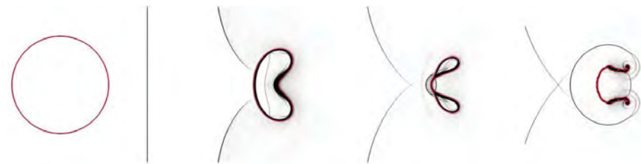
Fig. 12. Computed interaction of a shock wave with a cylindrical air bubble in water. Time progresses from left to right as a Mach 1.02 shock wave propagates from right to left. The shock initiates bubble collapse and a reentrant jet forms. When the reentrant jet collides with the distal side of the bubble, a secondary shock wave is formed.
