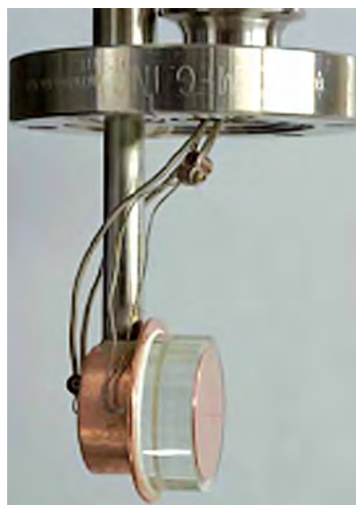
Fig. 3. Lithium iobate crystal mounted on a heater/cooler. A tungsten tip is attached to a copper electrode that is fixed to the surface of the crystal.
