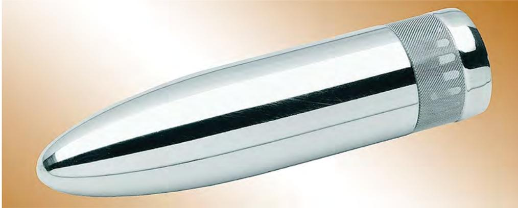
The Vibration Division of PCB® Piezotronics, Inc. introduces a new accessory model to its acoustic product line. Model 079B21 is a Nose Cone designed to be used with 1/2” (6 mm) condenser test and measurement microphones. The 079B21’s aerodynamic shape is designed to minimize noise due to wind and other high-speed laminar flows, while permitting the sound
