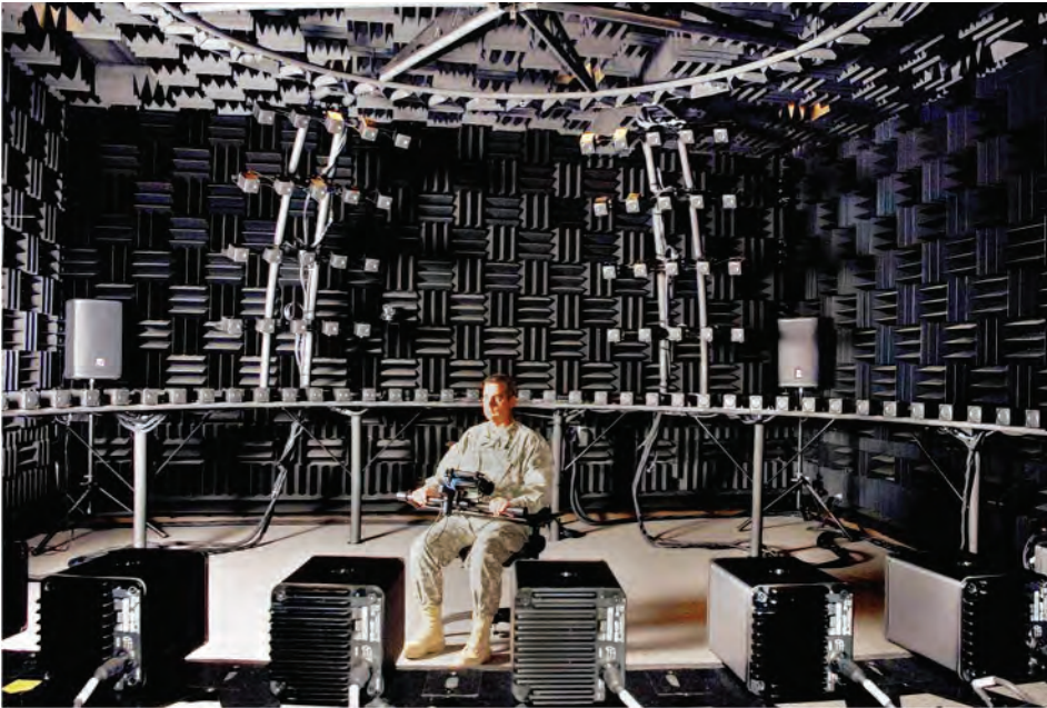
Fig. 4. A participant seated in the listener station of the Dome Room. The dense population of the loudspeakers in this room allows for precise measurement of auditory localization.
