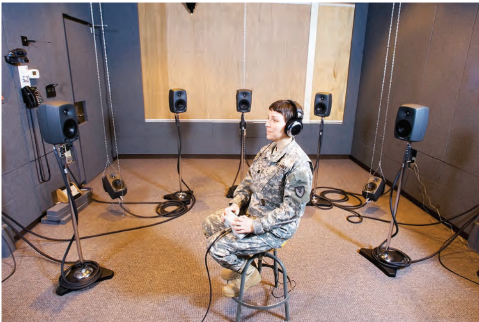
Fig. 6. A soldier listens to speech presented through headphones in the Listening Laboratory. The foam panels within this space can be removed to increase the reverberation time of the space.
