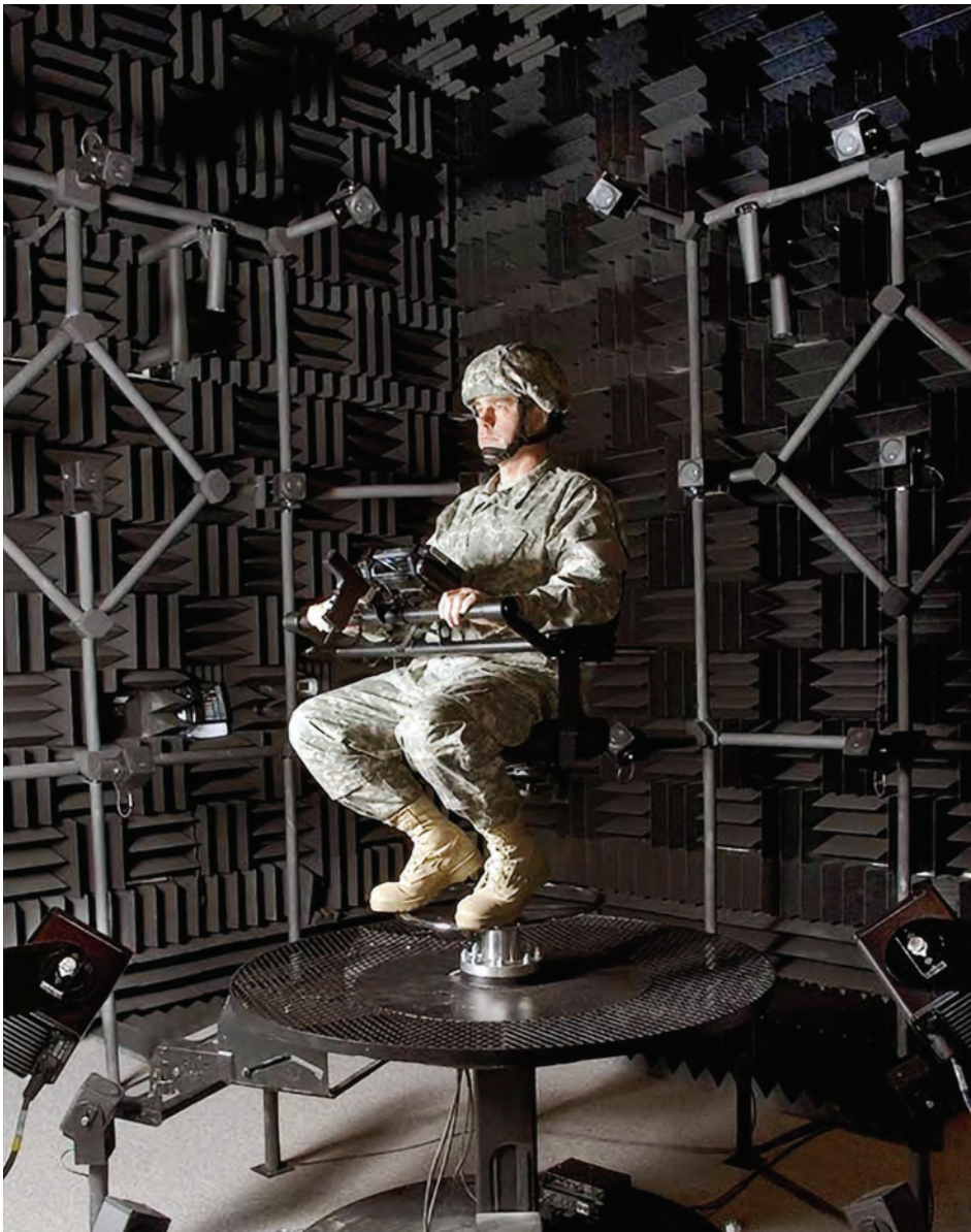
Fig. 3. A participant prepares for an experiment in the Sphere Room. The central location of the listener station and platform allow for the creation of a completely immersive auditory environment.
