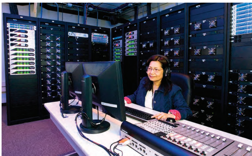
Fig. 2. A researcher configures an experiment in the Control Room. Rack mounted equipment is used to control the stimulus presentations in the research spaces.
