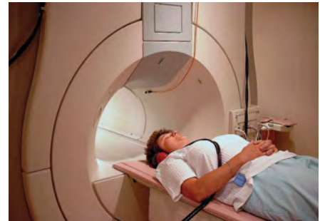
Fig. 5. Application of the optical microphone in the high-Tesla area of an MRI scanner for patient communication purposes.
