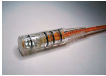
Fig. 3. Pre-production sample of the optical microphone. The diameter of the microphone is 1/2 inch.
