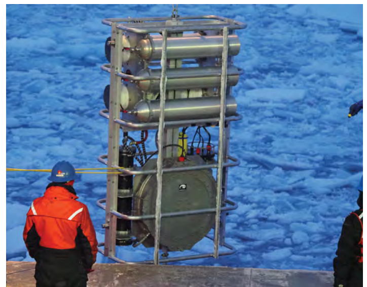
Figure 8. An ultralow-frequency source assembly ( f_0 = 35 Hz; \Delta f = 4 Hz) on the US Coast Guard Cutter (CGC) Healy during deployment in the Canada Basin during September 2019. The source transducer, developed by GeoSpectrum Technology, Inc., is mounted at the bottom of the frame. It is approximately 1 meter in diameter and 0.2 meter thick. Above it are high-pressure gas bottles for the pressure-compensation system needed to keep the internal gas pressure equal to the external water pressure. The pressure compensation system itself as well as the source controller, power amplifier, and batteries are on the opposite side of the frame. Photo by Lee Freitag, Woods Hole Oceanographic Institution, Woods Hole, MA.
