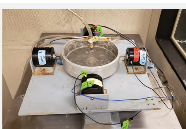
Figure 3. Dick’s original shaker table with four vibrators ( black ) moving the dish in which the fish is placed in the horizontal direction and a large vibrator under the table ( not visible ) moving the dish in the vertical direction. The table is still in use in the lab of Joe Sisneros (University of Washington, Seattle). Picture courtesy of Joe Sisneros.
