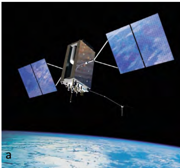
Figure 1. a: Image of Global Positioning System (GPS) III satellite. A GPS III satellite is roughly the size of a small car and orbits approximately 20,200 km above the earth. b: Configuration of satellite constellation. The original constellation contained 6 orbitals with slots for 4 satellites each, and only 24 satellites are required to operate at any given time. But, in 2011, this was expanded to accommodate additional satellites to improve coverage. Source: United States Government (available at gps.gov/multimedia/images ).
