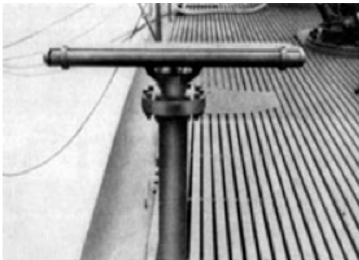
Figure 7. JP directional hydrophone, the fleet's first wideband surveillance system in the audio band.
