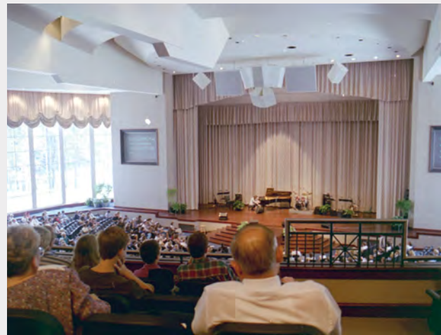
Figure 3. Recesses in the ceiling of the Perimeter Church north of Atlanta, Georgia, are actually “windows” coupling the main sanctuary volume with a reverberation chamber between the ceiling and the roof.
