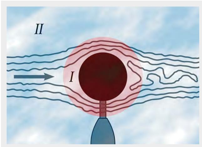
**Figure 3.** Diagram of a screened microphone in atmospheric turbulence. Streamlines illustrate the stagnation and distortion of flow around the windscreen. The sources for stagnation pressure are localized to region I (red), whereas the intrinsic pressure sources dominate in region II (blue).
