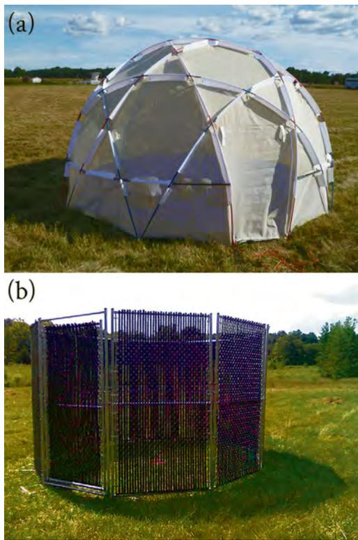
**Figure 8. a:** Photograph of a porous dome windscreen from Noble et al. (2014). Photograph courtesy of John Noble. **b:** Photograph of a wind fence (Abbott et al., 2015). Photograph courtesy of John Paul Abbott, with permission of the Acoustical Society of America.
