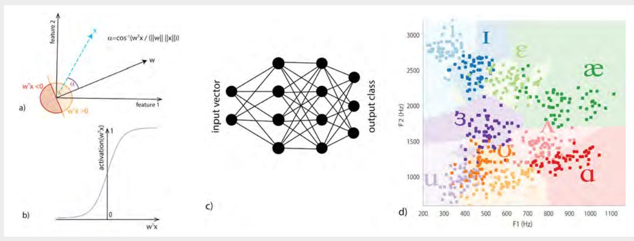
The dot product is then transformed (**Figure 3b**) by a differentiable nonlinear function called an activation (e.g., a sigmoid function or one that sets negative values to zero). Nodes are arranged into layers, and in a classic feed-forward network, the outputs of one layer serve as inputs to the next layer (**Figure 3c**). Thus, one can think about each node as making a local decision about which side of a hyperplane its inputs fall on and propagating this knowledge to subsequent nodes.
