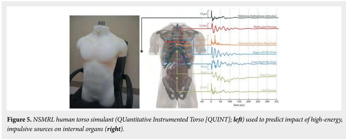
**Figure 5.** NSMRL human torso simulant (QUANTITATIVE INSTRUMENTED TORSO [QUINT]; left) used to predict impact of high-energy, impulsive sources on internal organs (right).
