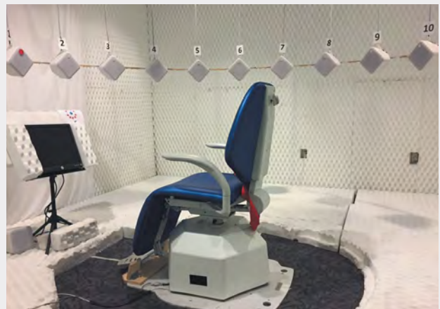
Figure 6. Bill's sound insulated room with rotating chair and surrounding speakers for studying auditory motion perception.
