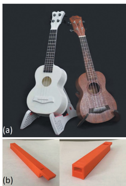
Figure 3. 3D-printed musical instruments. a: Printed ukulele (left) and wood instrument (right). Reproduced from Qian (2019), with the permission of the American Institute of Physics (AIP). b: A recorder that has been optimized using computer software (left) and a printed prototype (right). Reproduced from Thacker and Giordano (2021), with permission from the American Institute of Physics (AIP).
