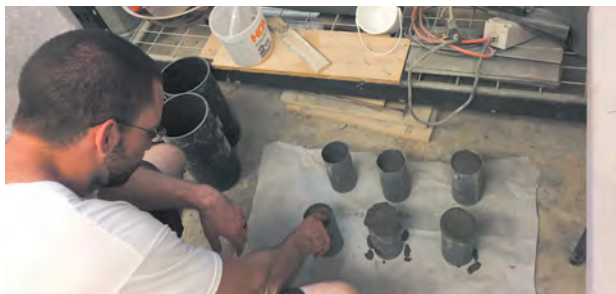
Figure 7. Top left: student developing concrete mixes in various size compression strength test cylinders. Top right: student placing acoustically diffuse and absorbent lightweight aerated concrete (ADALAC) panels in the Riverbank Acoustical Laboratories reverberation chamber. Bottom: close-up photographs of both the sawtooth ( left ) and recessed ( right ) prototype panels showing shapes and surface porosity responsible for reflection, diffusion, and absorption.
