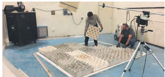
Figure 7. Top left: student developing concrete mixes in various size compression strength test cylinders. Top right: student placing acoustically diffuse and absorbent lightweight aerated concrete (ADALAC) panels in the Riverbank Acoustical Laboratories reverberation chamber. Bottom: close-up photographs of both the sawtooth ( left ) and recessed ( right ) prototype panels showing shapes and surface porosity responsible for reflection, diffusion, and absorption.
