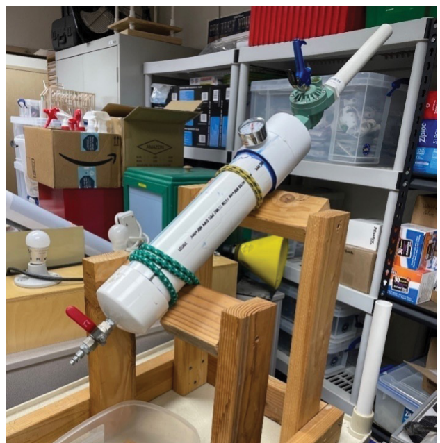
Figure 1. Two students in a pre-engineering class during their aerospace engineering unit with their exploded rocket (left) that was destroyed by the launcher (right). That launcher was powered by 60 psig (500 kPa) of air pressure to accelerate the rocket. The blue handle on the launcher actuates a quick-release valve.
