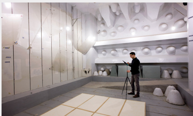
Figure 4. Reverberation chamber at the Technical University of Denmark, Kongens Lyngby. The chamber is equipped with hanging panel diffusers ( left ) and built-in boundary diffusers ( right ) to create a diffuse (mixed) sound field. Photo by Torben Nielsen.
