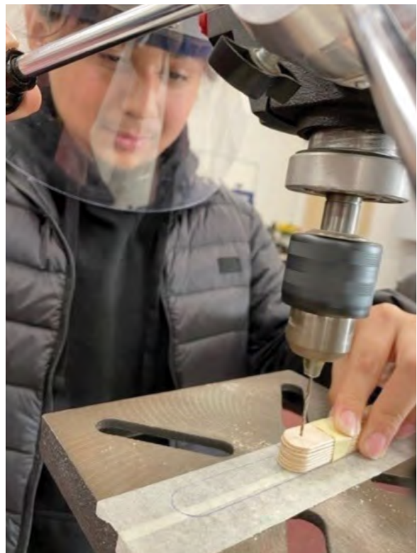
Figure 2. Top: hydraulically actuated scissor jack that uses two 10-ml syringes to raise and lower the jack. Bottom: a student is drilling the holes used as bearings (with copper wire) in all eight tongue depressors at once.
