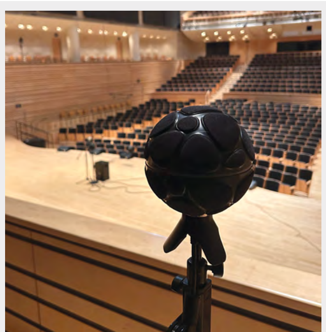
Figure 3. Example of a spherical microphone array. The black object has 19 microphone capsules embedded in a rigid body. For more information about the placement of the microphone capsules, design, and implementation of spherical microphone arrays, see Rafaely (2019).
