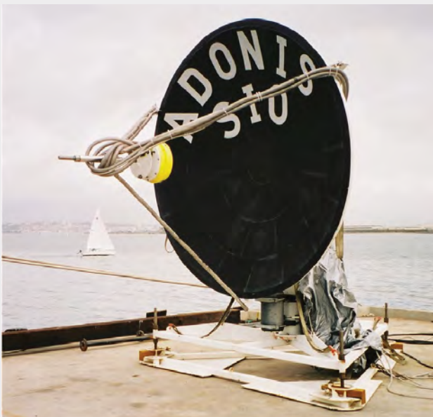
Figure 1. Acoustic Daylight Ocean Noise Imaging System (ADONIS) on the Scripps Institution of Oceanography Point Loma wharf, La Jolla, California. When placed in the ocean, the black spherical dish with a diameter of 3 m reflects and focuses underwater background noise onto the planar array of hydrophones ( yellow disc ). The dish and the array work together to create a spatial map of the noise field, arriving at the dish from different angles. This acoustic information is combined and visualized on a screen to produce images of objects in the ocean. Photo courtesy of the Buckingham Laboratory, used with permission.
