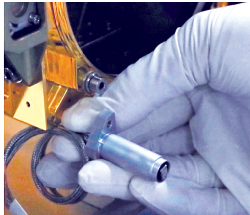
Figure 1. Left: SuperCam instrument on the Perseverance rover. Dashed red rectangle: microphone location. Right: microphone during its tests. It is 3.4 cm long and weighs a mere 13 g! Left courtesy of NASA/JPL-Caltech; right courtesy of ISAE-SUPAERO.
